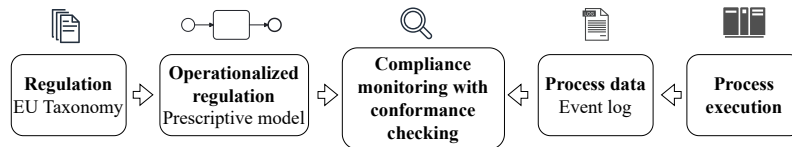
Fig. 1. Conceptual overview of compliance monitoring with conformance checking [7, 21]
